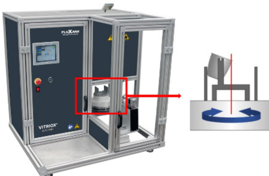
Figure 3: Rotation stirring principle in the VITRIOX® ELECTRIC
