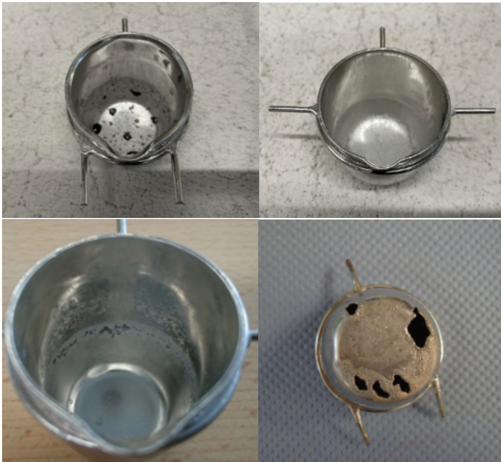
Figure 1: different types of damage to the crucible
