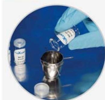
The customer receives a glass powder that contains a standard and flux. By directly filling the powder into the platinum crucible, a glass bead can be melted as a calibration standard for XRF without accurate weighing.
