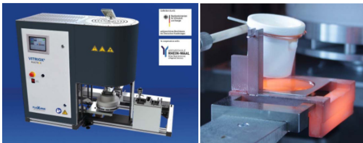
Figure 1: Electrical fusion machine with two stations; quartz crucible in use.
